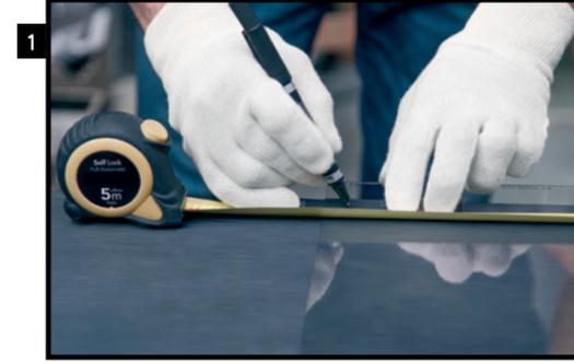
1 Cut the Artglass 99™ on the uncoated side of the glass.
