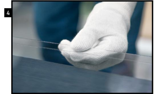
4 When you are using a manual glass cutter, place the UV-coated side on a clean, non-slippery, non-abrasive surface to avoid scratches on the surface.
